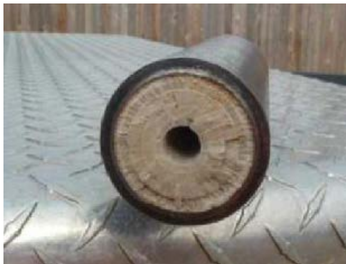
Figure D-16. Barium Sulfate Scaling in Haynesville Shale Pipe
